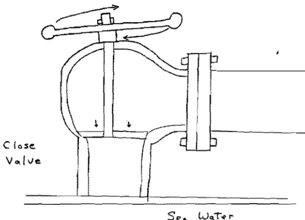
**Step Seven: Remove the retaining nut on the valve wheel.** You still need to reopen the valve but you need to remove the valve wheel quickly once you do so. You can remove it completely using your wrench, but the wheel is more efficient so leave it on for now. Check and make sure that it can be easily removed.
