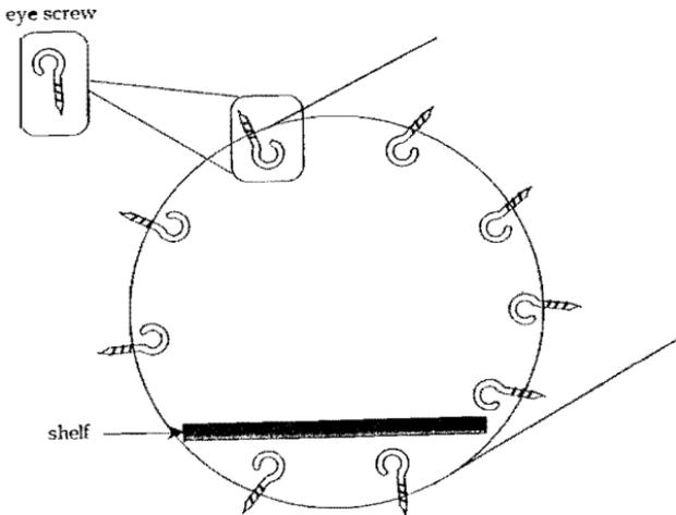
3) Corrugated roofing metal or other types of sheet metal are ideal materials for blocking culverts under roads. Use your ingenuity to affix them to the culvert so they will stay in place in high water. (Try using eye bolts as suggested above, or drive large nails into the walls of the culvert.)
