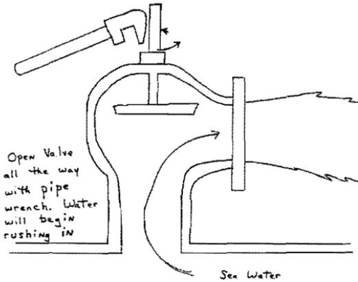
With your wrench, bash and bend the valve stem so that it will not be possible to close the valve.
